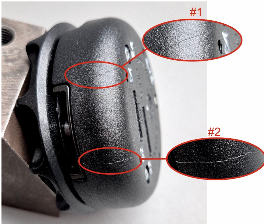
Picture 2: Acceptable Cracks – Class 1 and 2
