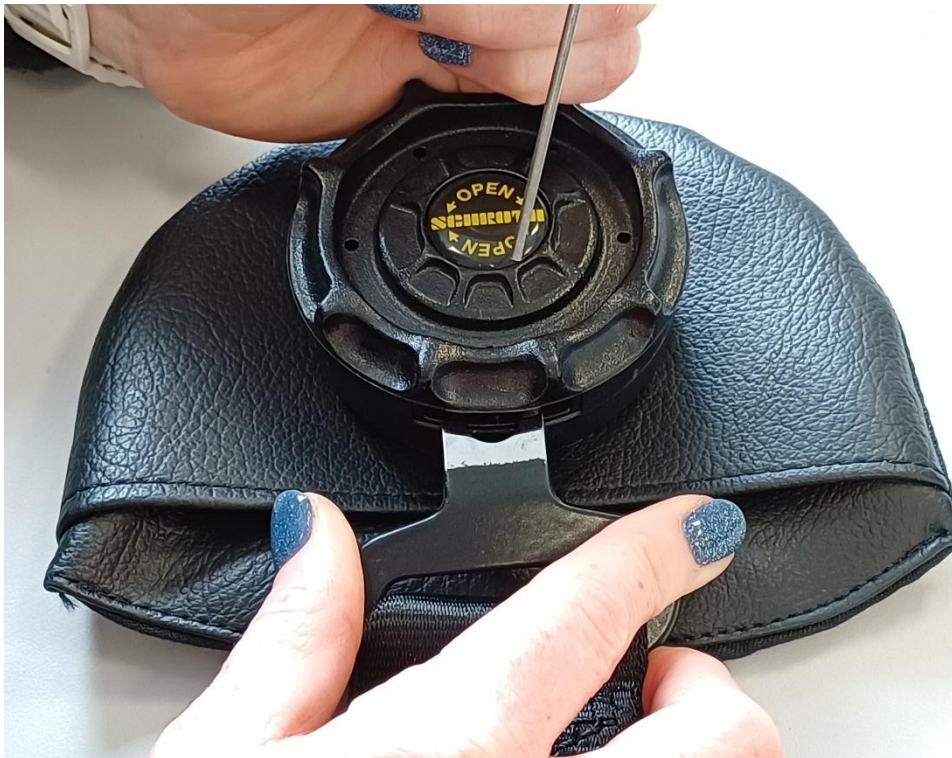
Picture 11: Insert Latch Completely
