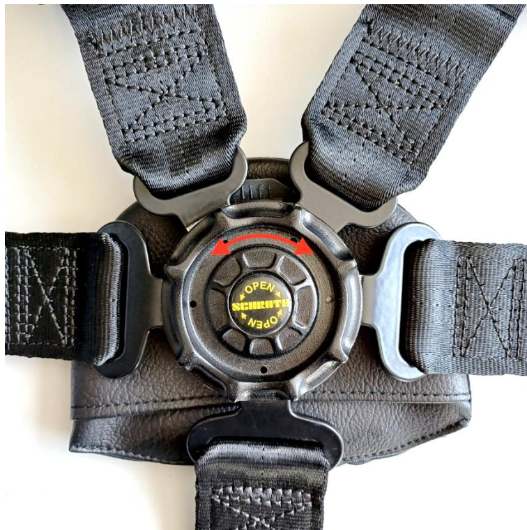
Picture 15: Rotate the Actuator to Eject the Latches
